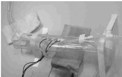
Fig. 19. A photograph of the pressure sensors for Pulse diagnosis and model circulation of a radial artery
