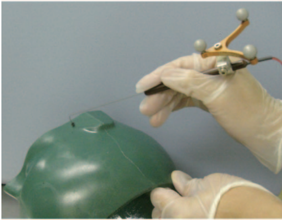
Fig. 10. Prototype microelectrode for human use Overall length of handle is 100 mm; the shaft section is also 100 mm. It uses a flat single channel bipolar electrode. An antenna for the 3D navigation system can be attached to the handle section. (*)
