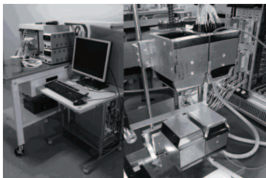
Fig. 10. Left is the PEM simulator. The PEM simulator is a subset of the PEM scanner and used for the diagnosis of the crystals and the PMTs. Right is a close up of the detector units.
