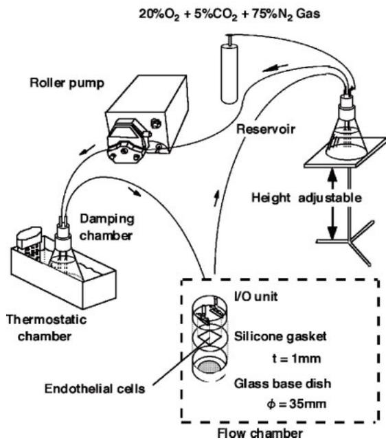
Fig. 1. Schematic diagram of hydrostatic pressure-imposed system. The height of the reservoir is manually changed to apply hydrostatic pressure to endothelial cell monolayer.
