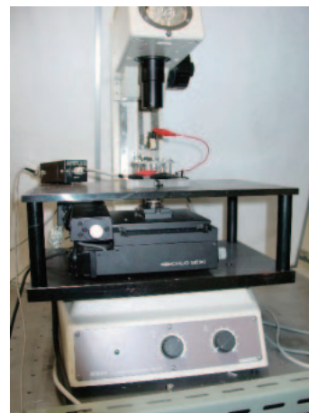
図5. Scanning system for the chemical imaging sensor.
